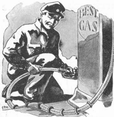
Rubber Washers Spaced Evenly on Gasoline-Pump Hose Protect It against Wear
