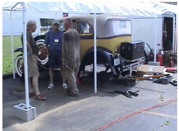
Above: H&H Engine Rebuilding giving the engine rebuilding seminar. Below: A car in the repair tent with the rear axle removed to get to the transmission for repair. Bottom: There was a good selection of spare parts if needed at the swap meet. Photos by Peter Crosby
