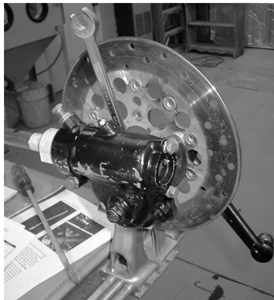
Steering box mounted in jig made from old motorcycle brake disk. (Yes I repainted the box after all this was over!)
